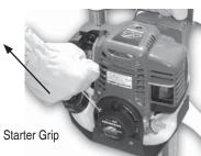
sistance, then with a swift motion pull the starter grip to start the unit. Gradually move the choke lever to the open position as the engine warms up. Do not throttle the driver when not seated on a post as it will damage the unit. continued on back...
